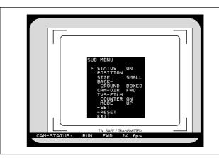
Like all man-readable information, the data is inserted as a window on the monitor image. The window can be switched on and off independently. Background, position and character format can be altered without affecting the settings of other windows.
