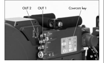
The "normal video" output (OUT 1) supplies almost no inserted electronic information. Only a flashing bar at the button left corner of the video image indicates a running film camera.
