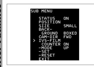
The sub menu line **IV5 FILM COUNTER** switches the IVS film counter on and off.
