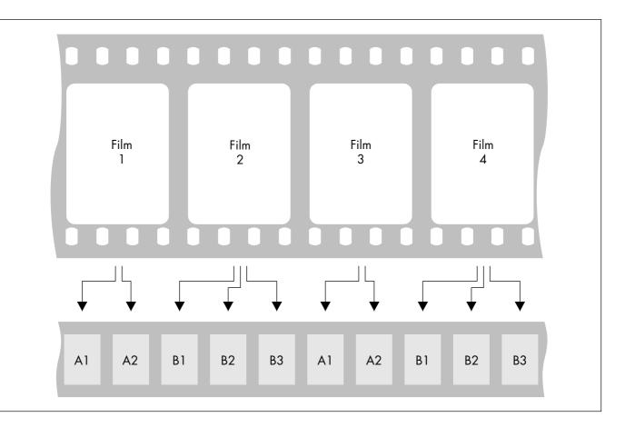
All video assists are based either on PAL or NTSC video systems, with a fixed video frequency of either 25 full video frames per second with PAL or 29.97 full video frames per second with NTSC. The speed of the film camera can however be selected over a wide range. At every film speed which is different from the video frequency, the IVS has to add repeated video fields to compensate for the different frame rates.
